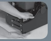
Floating vacuum shoe follows the contour of the carpet for superior recovery.
